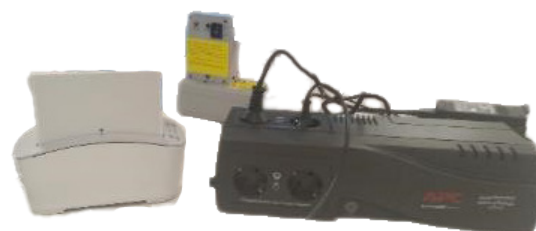
Battery chargers for Delft Light generator and detector
