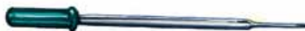
A simple air brush made using a Pasteur pipette and rubber bulb
